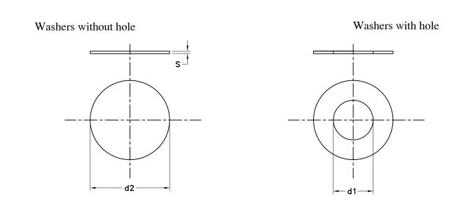
For a washer : d1=6.5 mm - d2=16.5 mm and S=0.5 mm from galvanized zn 8 bk c C (A3G)
